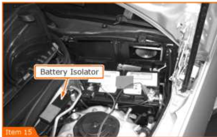
Fuse/Relay Box 2 - Incorporates battery isolator
